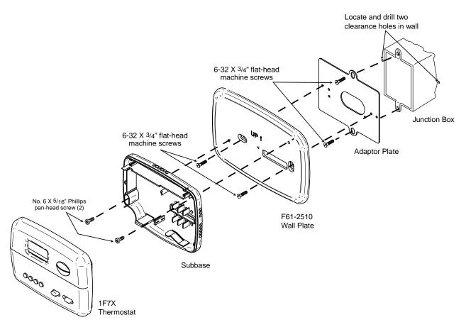
Figure 2. Mounting 1F7X digital thermostat to vertical junction box.
