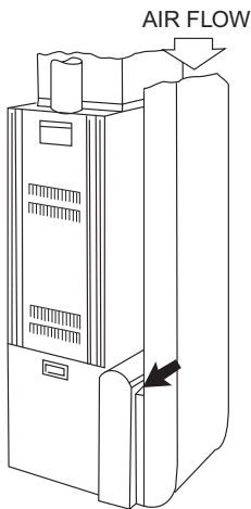
Figure 7 HIGHBOY FURNACE Side installation. Filter is mounted vertically, where return air enters side inlet of furnace.
