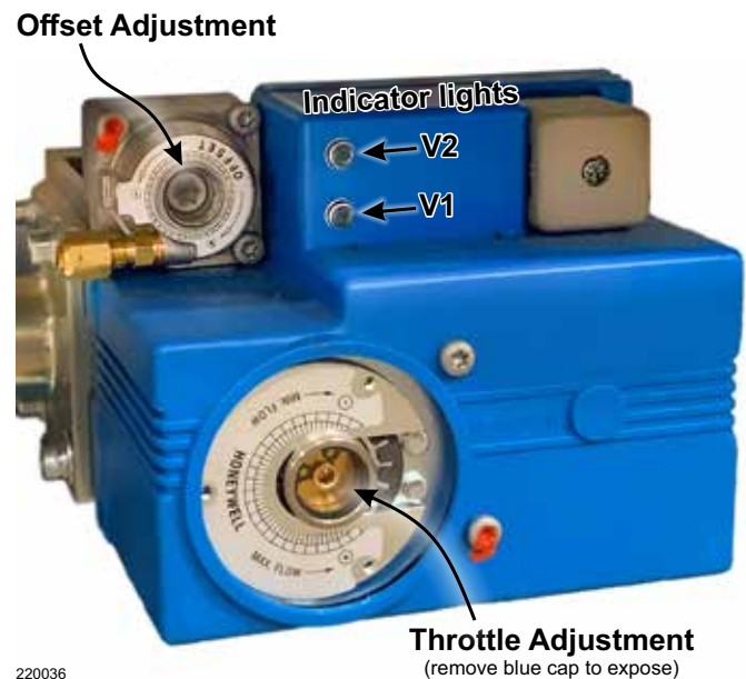
Figure 64 Throttle and offset regulating screws
