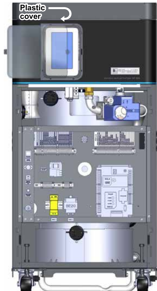
Figure 58 Protective plastic cover over touchscreen
