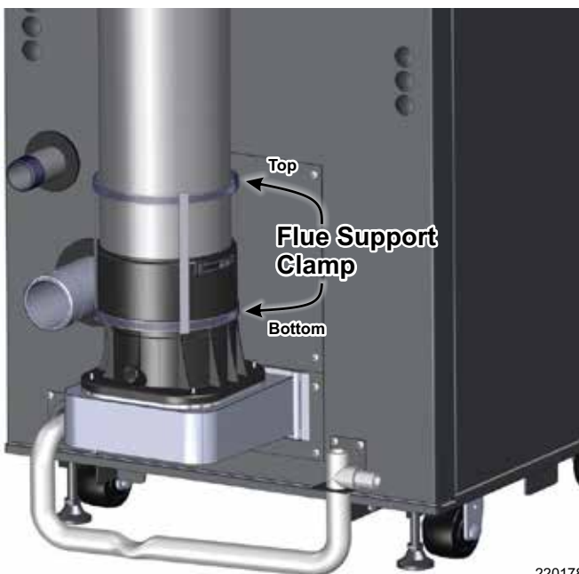
Figure 20 Flue support clamp, installed
