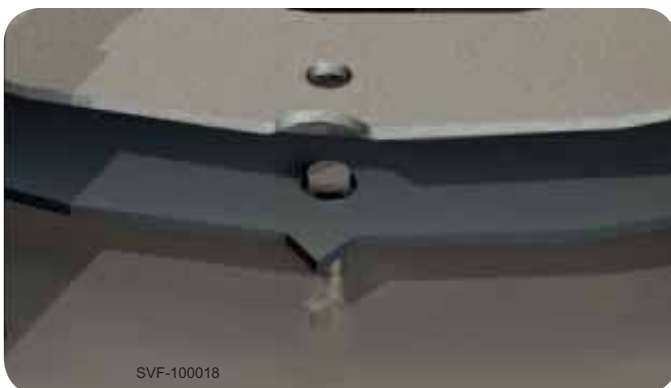
Figure 92 Burner and gasket with alignment orientation shown
