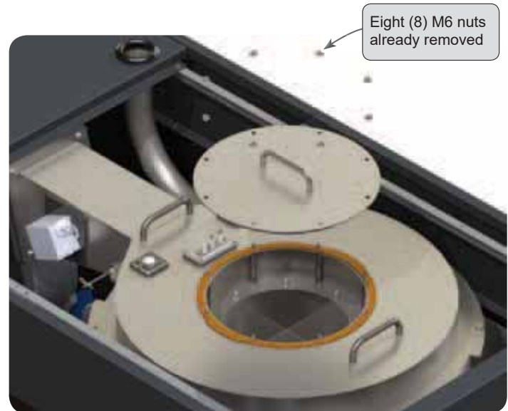
Figure 88 Access plate up for burner removal and replacement
