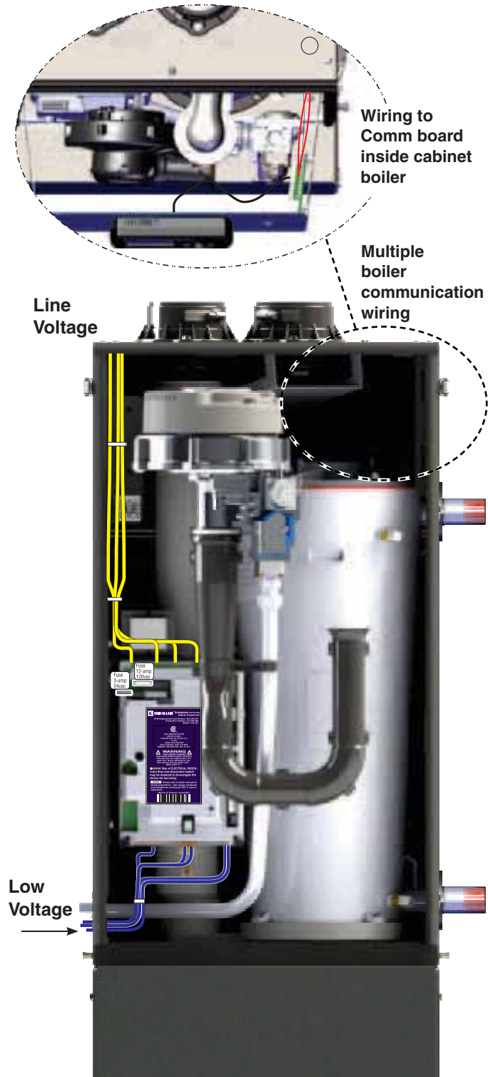
Figure 14 Field wiring overview (see Figure 15, page 34 and Figure 16, page 35 for detailed schematic and ladder wiring diagrams)
