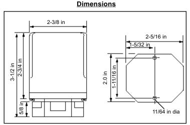
Use copper (60/70 $^{\circ}$  C) wire only. Torque to 20 inch pounds.
