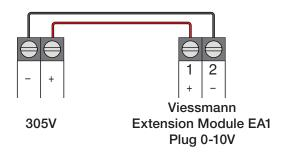
Connect to the Viessmann Extension Module EA1 Plug 0-10V.
