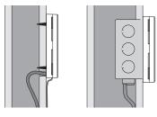
The enclosure is either mounted flush onto a wall or it can be placed onto a 2" x 4" non-conductive electrical box. The mounting holes in the enclosure accept #6 screws. Wiring to the control enters the wiring chamber through the back or bottom of the enclosure.
