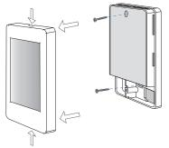
Grasp the front cover by the fingertip grips on the top and bottom of the enclosure and pull the front cover off.
