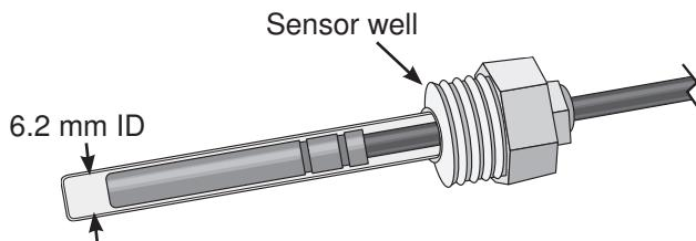
If a temperature well isn't available, the Solar Sensor 085 can be strapped directly to the pipe using a stainless steel clamp (not provided).
