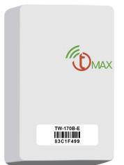
The MAX Range Encoder MDT has a true encoder interface that directly reads the meter face value of encoded meters to transmit an accurate reading towards the DCAP once per hour. The MAX Range radio has three to four times the range of our Standard Range MDT, which allows for far fewer or even zero Repeaters for faster system installations. It is ideal for manufactured housing or multifamily properties with limited Repeater installation locations.
