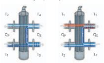
In this situation, demand is greater than supply. Some of the colder return water will join the supply, as a result of which it will take longer for the rooms to reach their set temperature. Where possible, the power of the boiler or chiller will then be increased.
