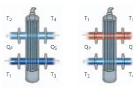
In this rare situation, supply and demand are exactly equal. This is the ideal situation in which the hydraulic separator operates primarily as a high efficiency air eliminator and dirt separator.
