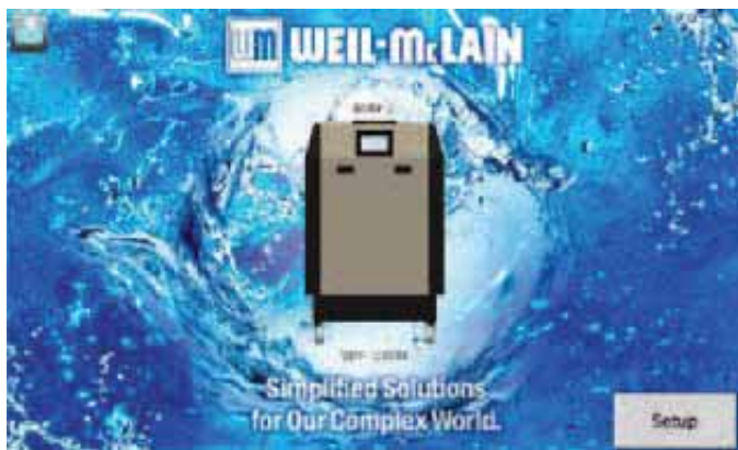
Figure 60 Sola display Home page (Single boiler system —boiler in normal operation)
