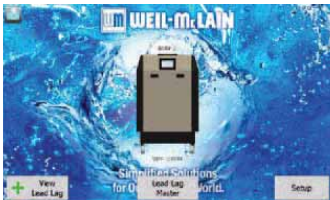
Figure 61 Sola display Home page (Boiler #1 in multiple boiler system —boiler in normal operation)
