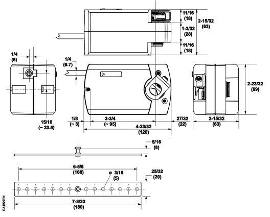
Figure 14. GQD1x1 Actuator and Mounting Bracket.
