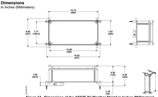
Figure 13. Dimensions of the ASK75.7U Weather Shield in Inches (Millimeters).
