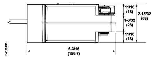
Figure 16. GQDxx6 with Conduit Adapter.
