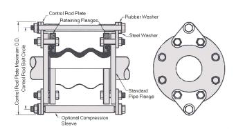
Technical Note: Flex-Weld strongly encourages the use of Control Rods in most, if not all, Rubber EJ applications. Most applications that utilize rubber expansion joints are not anchored properly. A simple pump connector does not protect against extreme stresses and strains produced by water hammer or air induced surge pressure, common to most applications, which greatly exceed normal system operating pressure.
