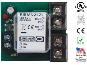
**Coil Voltage Input:** 24 Vac/dc ; 50-60 Hz Drop Out = 2.1 Vac / 3.8 Vdc Pull In = 18 Vac / 22 Vdc
