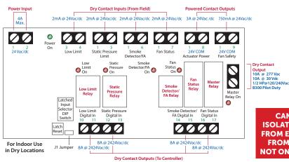
**CAN BE USED TO ISOLATE FIELD DEVICES** FROM EACH OTHER AND FROM CONTROLLER,
