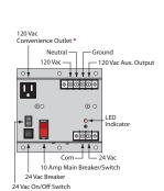
\* Move internal jumper to "HOT" position if you wish outlets to always be hot otherwise outlets will be switched by main breaker.
