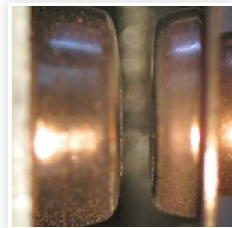
NOsparc ® PROTECTED CONTACTS 1 MILLION CYCLES
