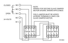
Fig. 5. Wiring five-wire control panel with additional slave damper.
