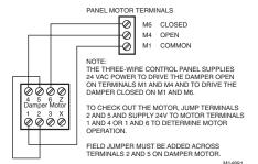
Fig. 2. Wiring a single damper from a three-wire control panel.
