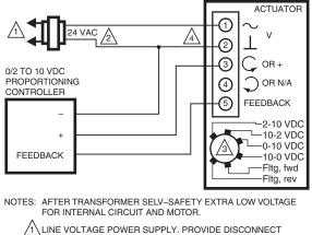
1 LINE VOLTAGE POWER SUPPLY. PROVIDE DISCONNECT MEANS AND OVERLOAD PROTECTION AS REQUIRED.
