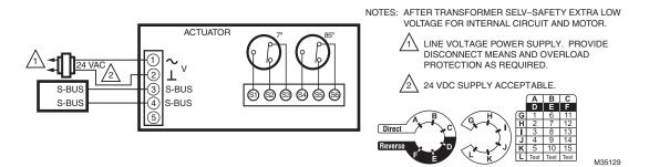
Fig. 25. Wiring for Sylk BUS, MS31 series.
