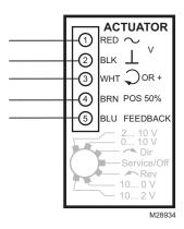
Fig. 29. MS7510W2008/2206; MS7520W2007/2205 Floating Modulating.
