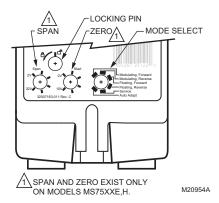
Fig. 4. Dials for control signal and zero/span.
