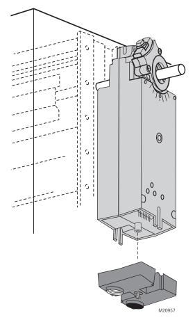
Fig. 10. Removing access cover.
