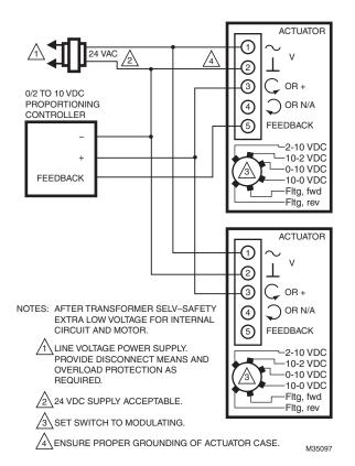
Fig. 24. Wiring for 0/2-10 Vdc modulating controller operating multiple actuators.
