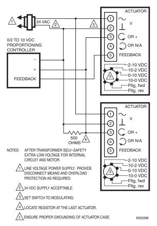
Fig. 26. Wiring for 4-20 mA modulating controller operating multiple actuators.
