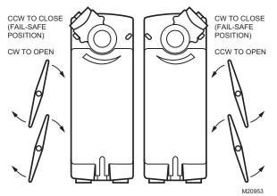
Fig. 2. Spring Return DCA mounting orientation.
