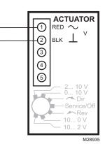
Fig. 30. MS8110W1008/1206; MS81200W1007/1205 Two Position Low.
