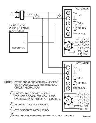
Fig. 27. Wiring for 0/2-10 Vdc modulating controller operating multiple actuators as master/drone.
