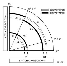
Fig. 34. SPDT End Switch Operation.
