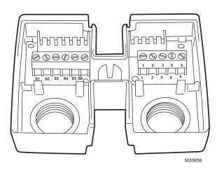
Fig. 11. Terminal block details.
