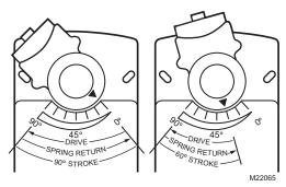
Fig. 6. Stroke reduction.
