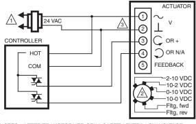
NOTES: AFTER TRANSFORMER SELV–SAFETY EXTRA LOW VOLTAGE FOR INTERNAL CIRCUIT AND MOTOR.
