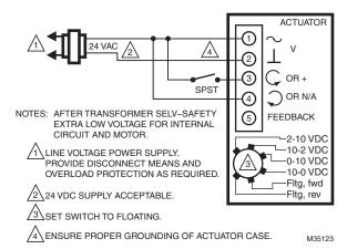
Fig. 16. Wiring for SPST on/off control.
