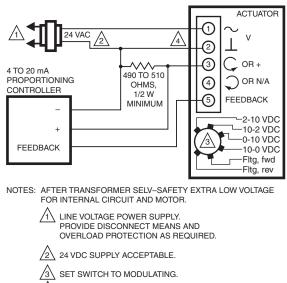
Fig. 20. Wiring for 4-20 mA modulating controllers.
