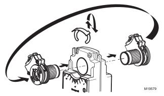
Fig. 3. Mounting shaft coupling to actuator opposite side.
