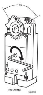
Fig. 7. Manual positioning.
