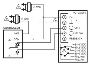
NOTES: AFTER TRANSFORMER SELV-SAFETY EXTRA LOW VOLTAGE FOR INTERNAL CIRCUIT AND MOTOR.
