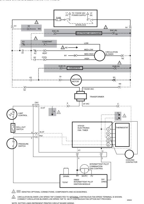
Fig. 5. ST9120U internal schematic for Intermittent Pilot application.
