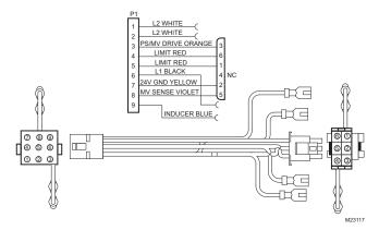
Fig. 7. ST9101 Wire Adapter Schematic
