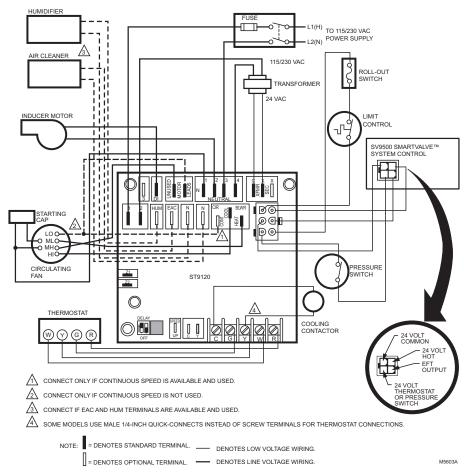
Fig. 2. Typical ST9120U wiring connections with SV9500/SV9501 SmartValve™ System Control.
