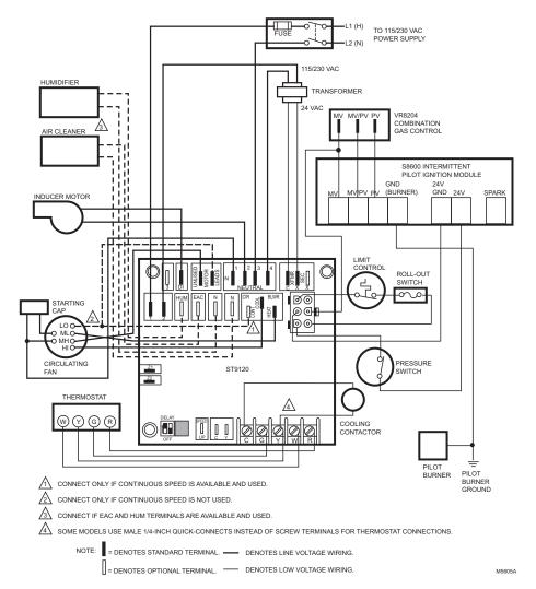
Fig. 1. Typical ST9120U wiring connections with S8600 Intermittent Pilot Ignition Module.
