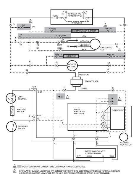
Fig. 6. ST9120U internal schematic for SmartValve™ System applications.
