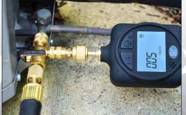
Easily attach and protect vacuum gauge with the slide valve side port
