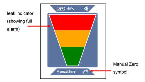
Manual Zero mode looks and operates similar to Pinpoint mode, but is identified by the text Manual Zero and the Manual Zero symbol on the bottom bar. Manual Zero mode allows the user to manually zero to the background refrigerant by pressing the SENS/ZERO button. Once the new zero point is set, D-TEK Stratus will not alarm unless a higher concentration of refrigerant is detected.
