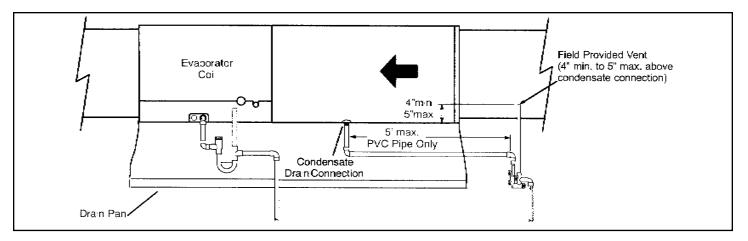
Figure 36. GUH97M with Evaporator Coil Using a Separate Drain (Unit shown in horizontal Left hand discharge position)
