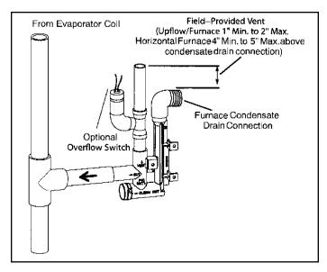
Figure 40. Condensate Trap with Optional Overflow Switch
