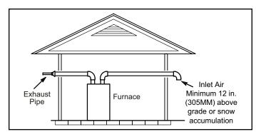
Figure 23. Exiting Exhaust and Intake Vent (no common pressure zone)
