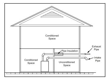
Figure 17. Insulating Exhaust Pipe in an Unconditioned Space
