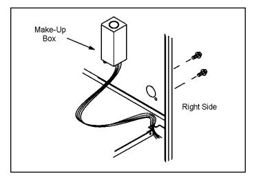
Figure 46. Interior Makeup Box Installation
