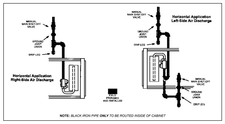
Figure 43. Horizontal Applications Possible Gas Piping Configurations
