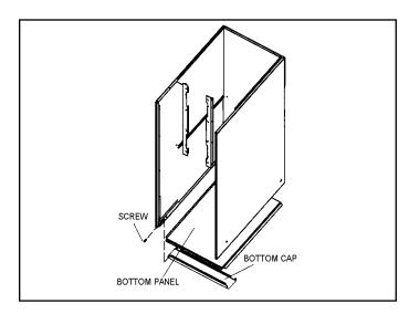
Figure 7. Removing the Bottom Panel
