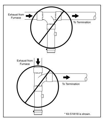
Figure 31. Crawl Space Vent Pipe Drain Trap
