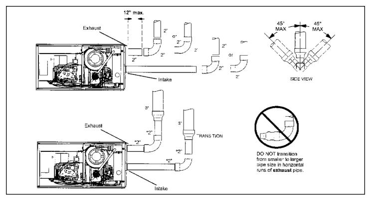
Figure 19. Typical Exhaust Pipe Connections and Condensate Trap Installation in Horizontal Air Applications (Right Hand Discharge Shown)
