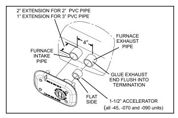
Figure 27. Flush-Mount Side Wall Termination 51W11
