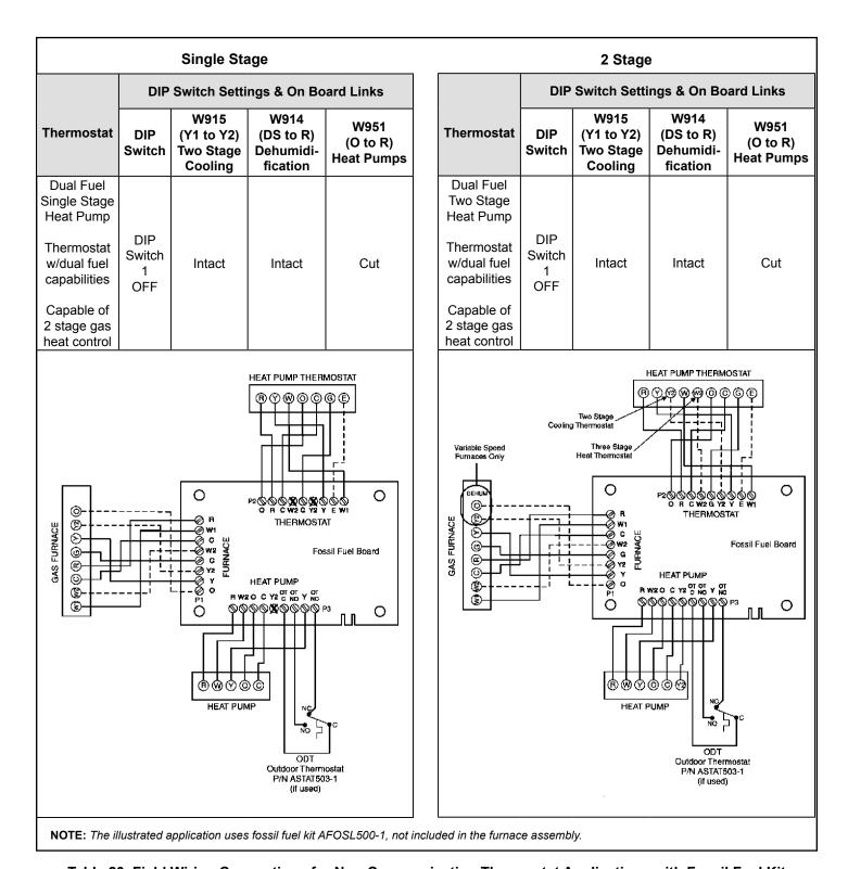
Table 20. Field Wiring Connections for Non-Communicating Thermostat Applications with Fossil Fuel Kit
