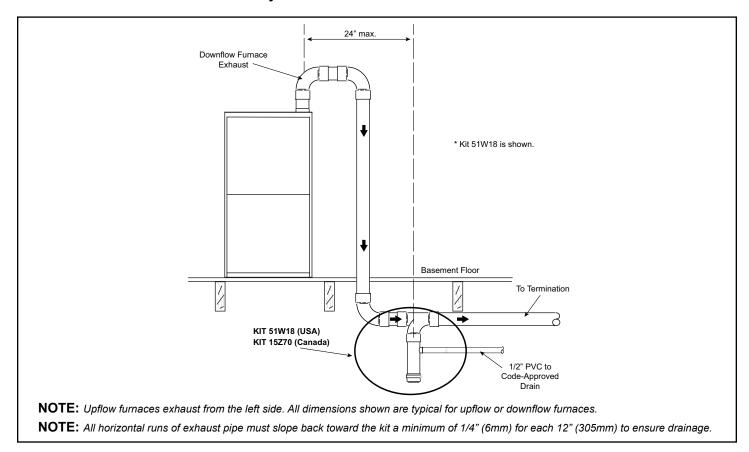
Figure 32. Upflow or Downflow Furnace with Exhaust through Crawl Space
