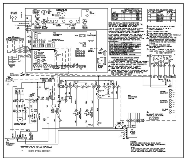
Figure 50. Typical GUH97M Wiring Diagram
