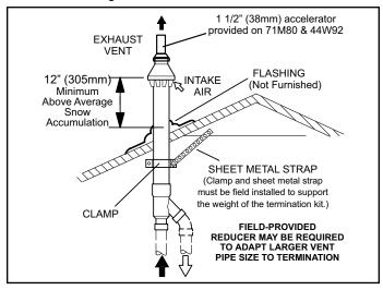
Figure 25. Direct Vent Concentric Rooftop
