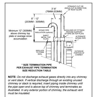
Figure 26. Direct Vent Application Using Existing Chimney
