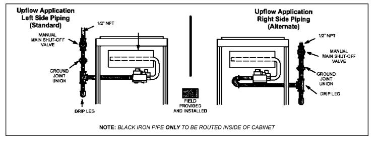
Figure 42. Upflow Applications Possible Gas Piping Configurations
