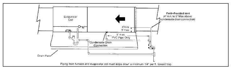
Figure 39. Evaporator Coil Using a Common Drain (Unit shown in Horizontal Left-Hand Discharge Position)
