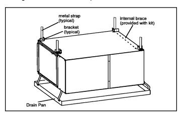
Figure 12. Typical Horizontal Application
