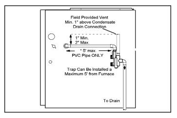
Figure 34. Condensate Trap Locations (Unit shown in upflow position with remote trap)
