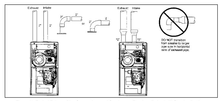
Figure 18. Typical Exhaust Pipe Connections and Condensate Trap Installation in Upflow Applications
