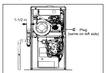
**NOTE:** In upflow applications where side return air filter is installed on same side as the condensate trap, filter rack **MUST** be installed beyond condensate trap or trap must be relocated to avoid interference.
