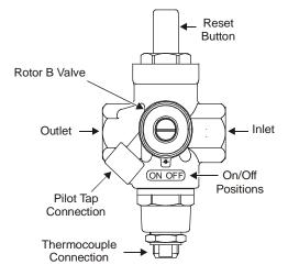
Figure 3: Typical H19 Valve with Rotor Valve
