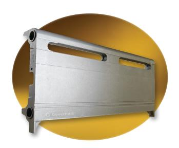
Gov-Board cast iron baseboard style radiation offers an "almost invisible" installation. Durable cast iron will allow years of worry-free comfort and provides more than five times the amount of radiant heat than conventional thin metal baseboards. This is due to the fact that the combined cast iron surface area is much larger than that found on thin metal baseboards. Gov-Board baseboards also offer the advantage of being able to distribute heat in both horizontal and vertical directions.
