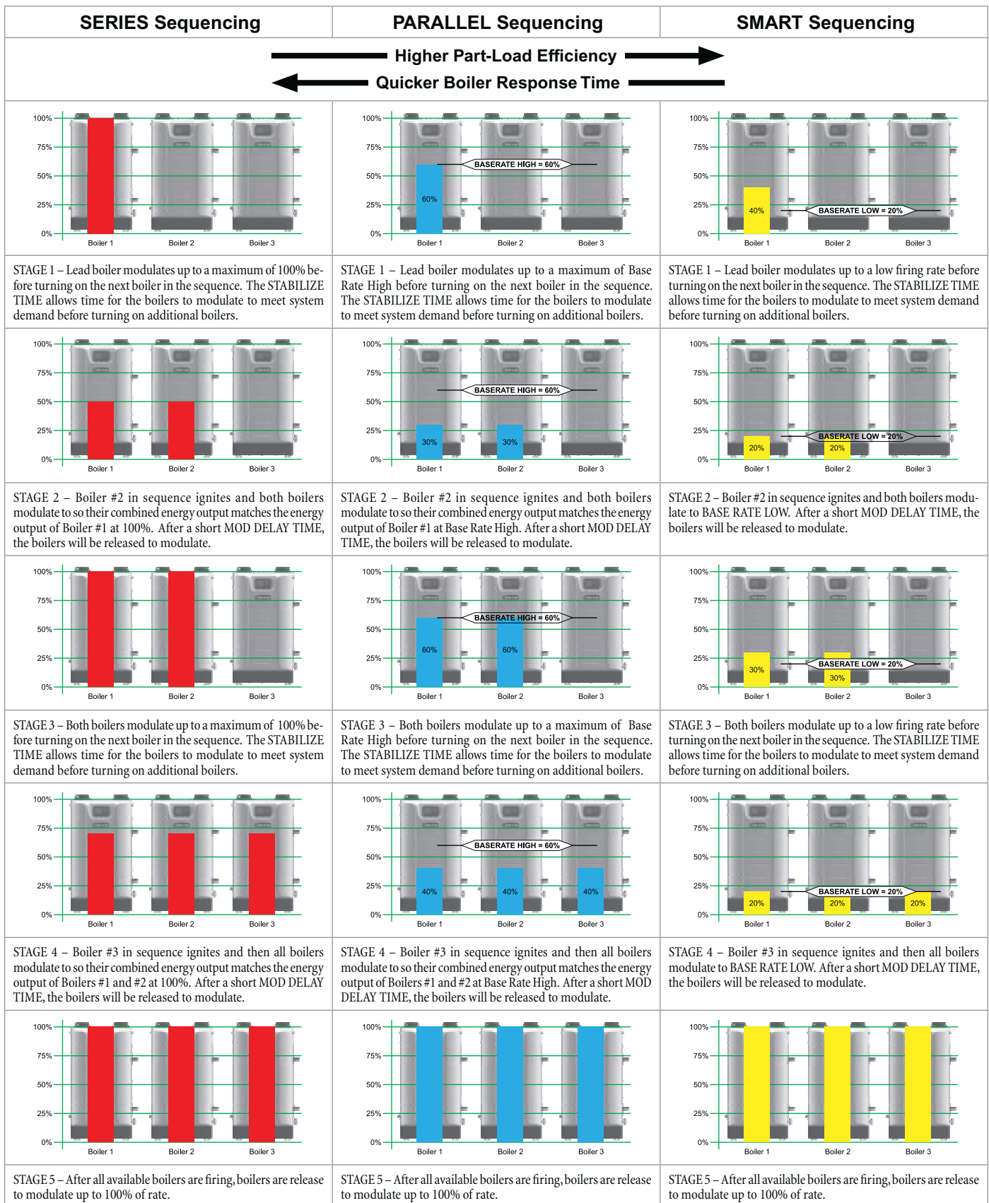
Figure 26 Evergreen sequencing options — SMART, PARALLEL or SERIES (examples shown for 3-boiler network)
