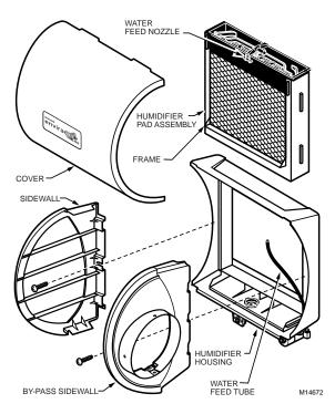
Fig. 5. Location of humidifier parts.
