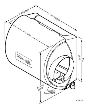
Fig. 1. Dimensions of HE225A,B in in. (mm).
