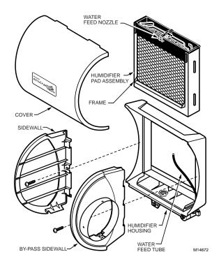
Fig. 4. Humidifier components.
