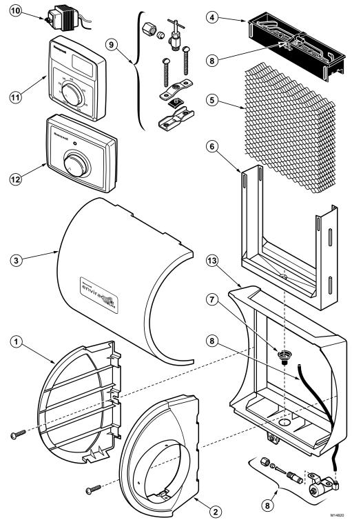
Fig. 6. Exploded view of humidifier parts.
