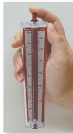
For high scale reading, finger covers hole
