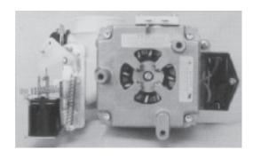
Note - On Electronic Drain Feedback switch models, install the adapter bracket (11) to the solenoid using the 2 screws
