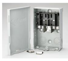
remove the two stainless steel hinge clips and move them to the righthand side. This permits the door to hinge on the right.
