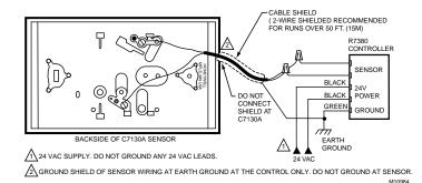
Fig. 3. General wiring hookup for C7130A sensor to R7380 Controller.
