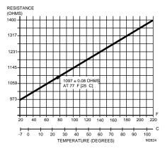
Fig. 5. C7130B resistance vs. temperature performance characteristics.
