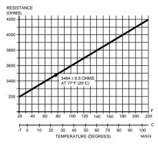
Fig. 4. C7130A Sensor resistance vs. temperature performance characteristics.
