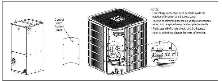
Figure 27 Low Voltage Unit Connections
