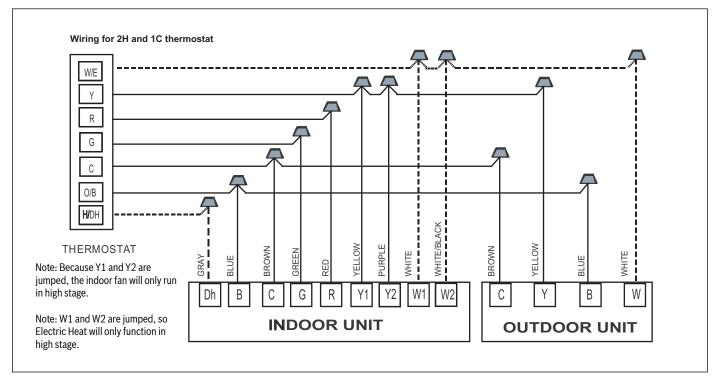
Figure 33 Thermostat Wiring Diagram for BOVB20/BVA20 Matched System
