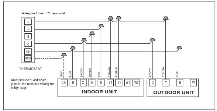
Figure 32 Thermostat Wiring Diagram for BOVB20/BVA20 Matched System
