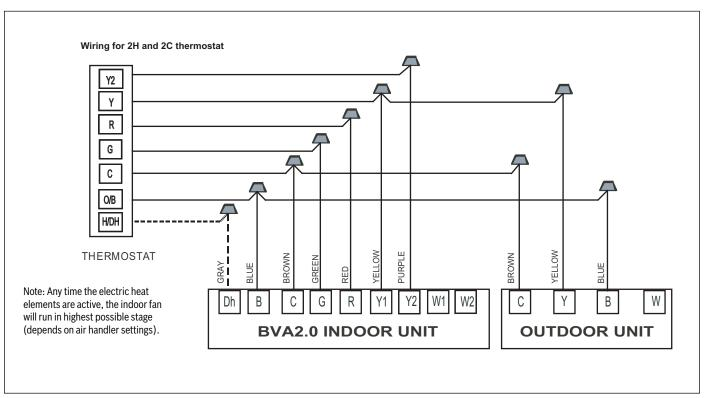
Figure 29 Thermostat Wiring Diagram for BOVB 18/BVA2.0 Matched System
