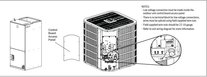
Figure 24 Low Voltage Unit Connections
