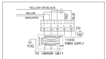
Figure 25 Wiring schematic example (refer to unit for actual wiring schematic)
