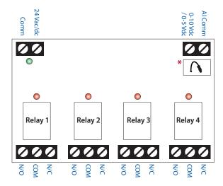
\*Must clip resistor in white box for 0-5Vdc.
