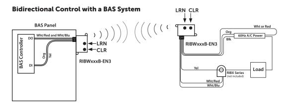
In this application the BAS system dry-contract output controls the transmitter on a RIBWxxxB-EN3. A second RIBWxxxB-EN3 receives the signal and activates it relay. A current switch detects current flow through the load and closes the dry-contract input on the second RIBWxxxB-EN3. The first RIBWxxxB-EN3 receives the transmission and closes its relay. This contact closure to the BAS system lets the controller know the load status.
