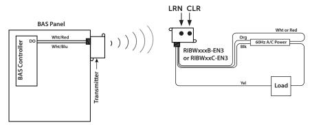
In this application the BAS system dry-contract output controls the transmitter and a RIBWxxxB-EN3 or RIBWxxC-EN3 is the receiver.
