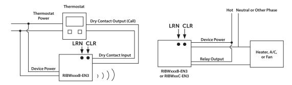
In this application the thermostat dry-contract output controls the transmitter and a RIBWxxxB-EN3 or RIBWxxC-EN3 is the receiver.
