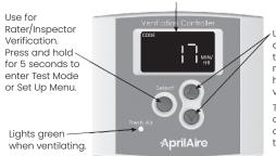
Use to override the calculated ventilation time setting (6 – 60 minutes/hr). Press and hold ▼ to turn ventilation OFF
