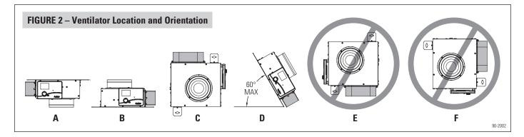
After deciding which orientation the ventilator will be installed, make sure the pivot of the backdraft damper is located above the centerline of the collar. Remove the outlet collar and rotate it 180° if needed to make sure the backdraft damper functions properly.
