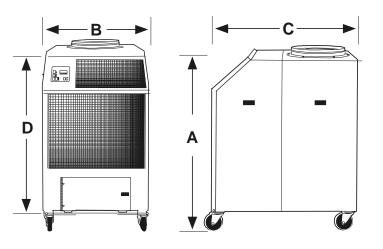
Note: Condenser inlet air plenum adds 13 inches to dimension "C"
