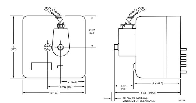
Fig. 1—Mounting dimensions of RA890 and R4795 Flame Safeguard primary controls with the 118702E in in. (mm).
