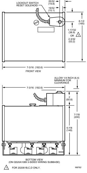
Fig. 4—Mounting dimensions of R7795 primary with 198365A,B,C remote reset cover, in in. (mm).
